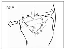
Move the cutter several times over the disc with the grinding movement (fig. 8). If the pendulum hook is too far inside, the cutter will rub on the upper side (fig. 9). If the
