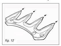
Check that you have a slight burr on the four tips of your cutter that move up or down when you touch them (fig. 12), check that the whole surface of the cutter is ground and there are no dull patches. If in doubt, grind it again.
